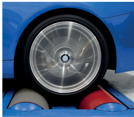
Any test rig requires a high dynamic load and negative torque on the motor shaft. The RFE allows for a very dynamic load in all four quadrants.
