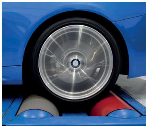
Any test rig requires a high dynamic load and negative torque on the motor shaft. The RHD allows for a very dynamic load in all four quadrants.
