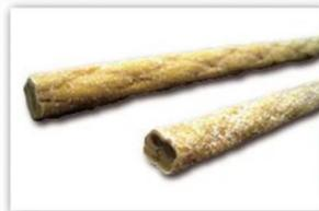
With silica sand on the surface, more adhesion to concrete and less occurrence of cracks. Using highly pure (99%) silica sand.
